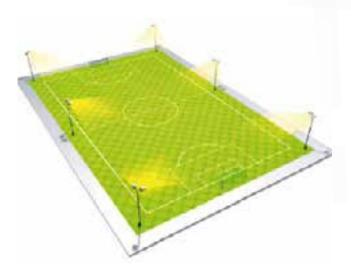
**Grade B – G (Steps 2-7)** Minimum FA standard for new installations 6 x 15m masts Average illuminance 200 lux (maintained)
