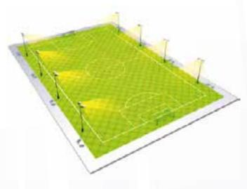
**3G Football Turf Pitches** 8 x 15m masts Average illuminance 200 lux (maintained) Modern lamp technology and designs have significantly improved the efficiency of lighting systems when compared with older installations with reduced running costs and improved spill control a major benefit. Floodlights fitted with Metal Halide lamps and using flat style optical systems are typically 30% more efficient than older asymmetric lighting systems.
