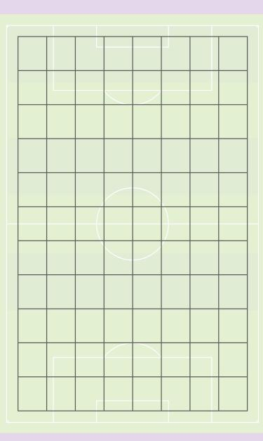
This grid must be submitted together with a signed Floodlight Inspection Report supplied by an approved lighting contractor. The position of the towers must be indicated on the survey chart.
