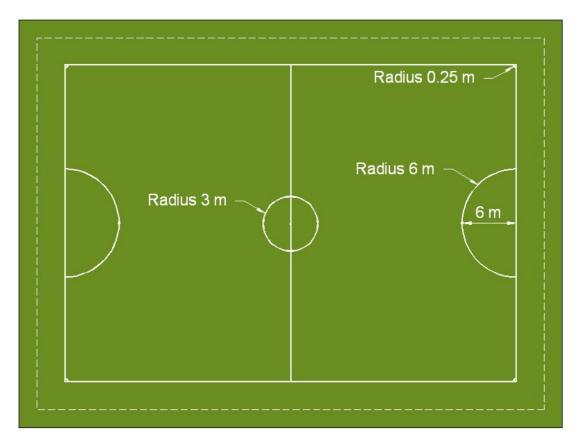
Figure 1 Markings for five, six and seven-a-side football (dotted line shows boundary of run-off where pitch is not enclosed)
