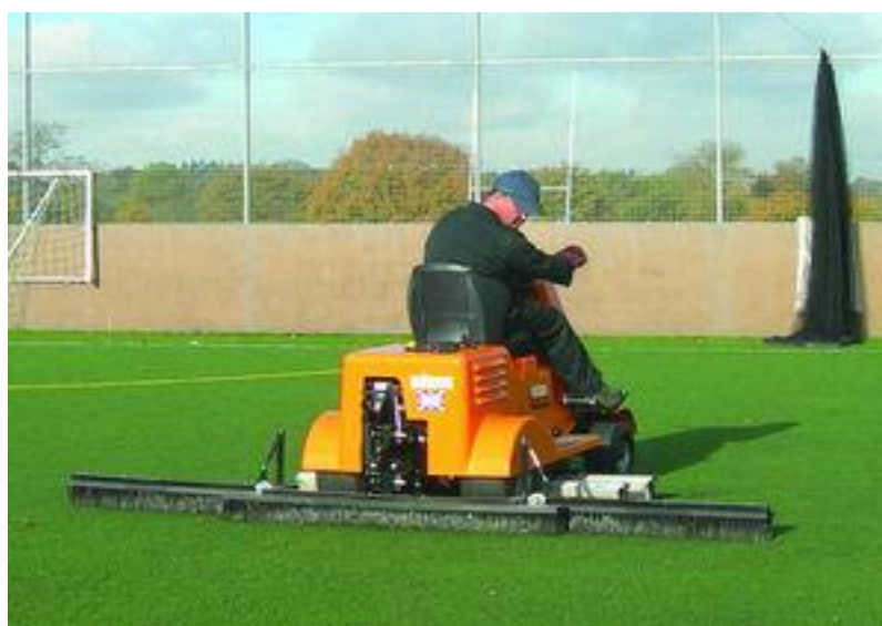
Ride-on brushing system with oscillating brushes
