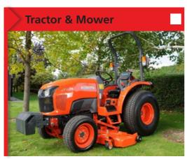
As above including mid mounted side eject cutting deck. The deck has 3 cutting blades with a cutting width of 152cm.
