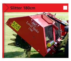
This Slitter allows air/water exchange to take place aiding drainage, this is a fast and proven method of aeration.
