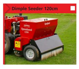
The Dimple Seeder is a popular way of applying seed to football pitches. The conical shaped spikes create a pocket in the soil which the seed is then dropped into. The rear roller the closes this pocket and ensures germination can take place. The metering wheel allows the seed rate to match travel speed.
