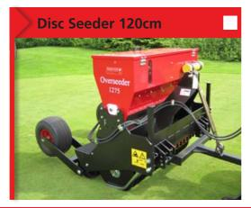
The Disc Seed will cut a groove into the surface, the disc then drops the seed to the bottom and closes the soil over the seed. The 1275 Overseed has easily adjustable application rates like the Speedseed and utilises a land - drive wheel to match seed rates to travel speeds.
