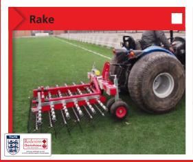
The Verti-Rake decompacts the turf surface using thin spring-loaded and flexible tines.
