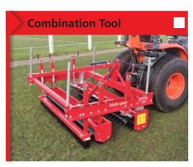
The Multi-Sport combination tool offers many features in one unit. The ability to slit, rake, roller or brush in pass to varying depths is invaluable to football surfaces. The storage stands make dismounting or mounting from the tractor very easy.
