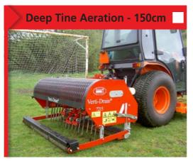
The Verti-Drain deep tine aerator is an invaluable tool for the aeration of football pitches. The 7215 Verti-Drain has an adjustable working depth and the option to add heave. There are a range of tines available depending on the requirements.
