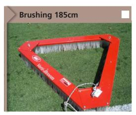
A triangular brush that can be towed by most prime movers. The unit can be pulled from any side to spread wear and maximise life span. The bristles stand up carpet fibre and move infill into site to support fibres.
