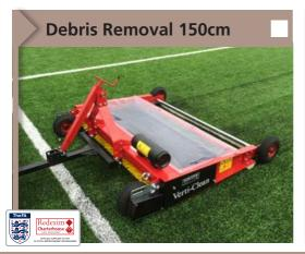
A land driven towed unit to collect surface dirt and debris from synthetic turf surfaces. The machine uses a rotary brush to flick material onto an oscillating sieve. The foreign material remains here for removal while infill is returned to the surface.
