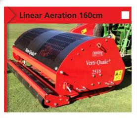
As with the Verti-Quake featured on page 10, the 2516 utilises rotary blade action to de-compact the soil profile. The 2516 has a larger working width at 160cm with the same maximum working depth of 250mm.
