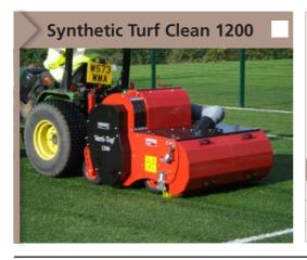
The Verti-Top utilises a powered brush to sweep into the carpet removing infill, dust and detritus. This material is then placed on an oscillating sieve to be separated from the infill to be returned. A vacuum system removes dust and fibres during the cleaning process.
