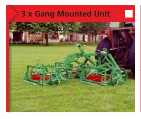
Linkage mounted cylinder mower gang. Land - driver cylinders will cut flat areas quickly. The units have 6 bladed 190mm diameter cylinders. The linkage mounted feature allows the whole machine to be lifted from the ground for transport or storage.
