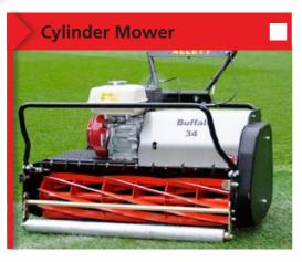
A self propelled Cylinder Mower, powered by a Honda engine. The cutting height can be adjusted from 10mm to 40mm. The machine comes with a grass collection box. This machine is only suitable for flat, level surfaces.
