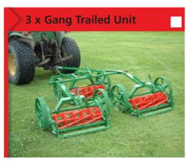
Towed gang unit - land driven. The cutting units have a 6 bladed 190mm cylinders for football surfaces. Only suitable for flat - debris free areas. The three units give a total cutting width of 230cm.
