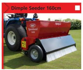
The larger 1600 Dimple Seeder allows for larger areas to be covered in one pass. The use of a seeder ensures that grass seed is drilled to germinate and not left on the soil surface.
