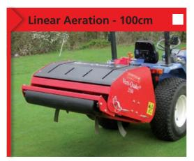
The linear process of aeration the Verti-Quake employs encourages root growth and shatters soil pans - with adjustable working depth the 2510 can be used around the year. The rear roller will stripe the surface as the machine passes over.
