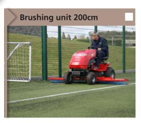
The RTC has been developed with regular brushing in mind. The self contoured unit allows for the routine maintenance to be carried out by one machine. With a working width of 200cm and a fold-able wings the RTC can be stored and accessed easily.
